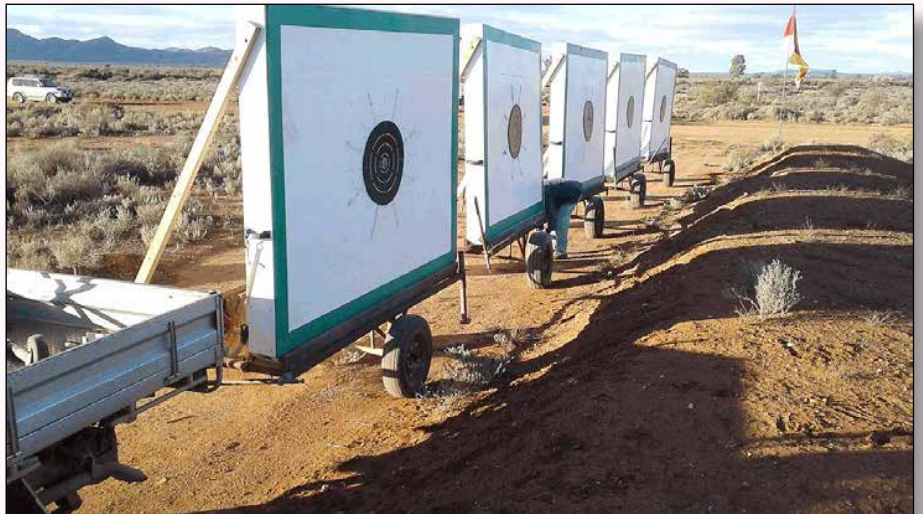
Yuntas Hexta targets are trailer mounted and towed to the different locations up the range, thus the shooters conveniently fire from the one mound all day - a much-admired innovation
